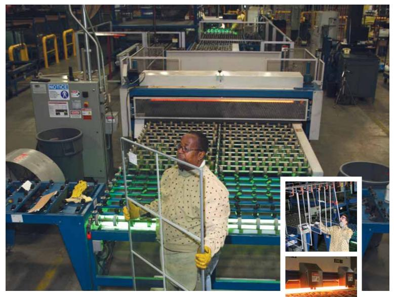
The Vitro Glass Residential IG Service Center can produce standard and triple-glazed IG units with tempered and low-e glass and incorporate Intercept spacer technology or flexible spacers.
